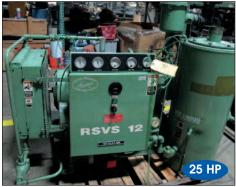
Sullair Rotary Screw Air Compressor Model RSVS-12-25AC
