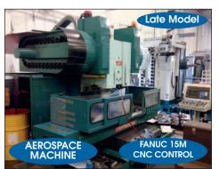
MATSUURA # MC-1000-VDC "Twin Spindle" CNC VMC
