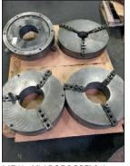
VIEW of "LARGE BORE" 3-Jaw Chucks
