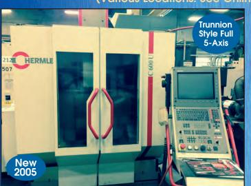
HERMLE # C-600U "5-AXIS" CNC VERTICAL MACHINING CENTER
