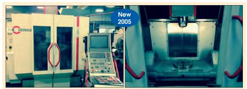
HERMLE # C-600U "5-AXIS" CNC VERTICAL MACHINING CENTER W/ "TRUNNION" STYLE "5-AXIS" ROTARY TABLE
