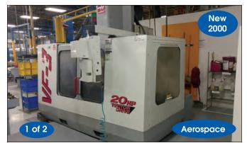
HAAS # VF-3 CNC VERTICAL MACHINING CENTER
