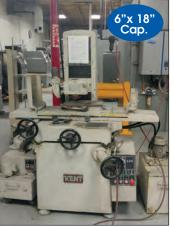
KENT # KGS-250-AH "HYDRAULIC" SURFACE GRINDER
