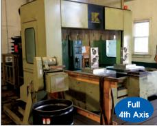
KURAKI # KH-80 CNC "4-AXIS" HORIZONTAL MACHINING CENTER
