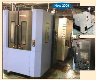
DOOSAN # HP-4000 "4-Axis" CNC Horizontal Machining Center
