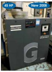
ATLAS-COPCO # VA-30VSD Rotary Screw Air Compressor
