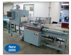
SHANKLIN L-SEAL PACKAGING MACHINE MODEL A-27A
