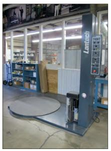
LANTECH ROTARY STRETCH PALLET WRAPPER, Q-SERIES
