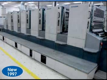
Komori 6-Color Sheet Fed Printing Press Model L640-III+C
