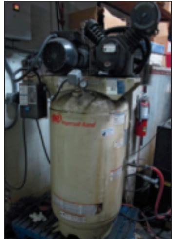
INGERSOL RAND 5 HP VERTICAL TANK AIR COMPRESSOR MODEL 2475
