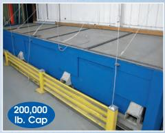
Navtec Hydraulic Pull Tester 200,000 lb. Cap.
