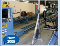
Navtec Fiber Winding Machine Model WBP-1-4-120-OMNIPC
