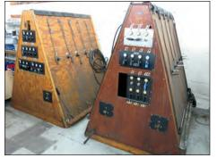
(2) NAVTEC A-FRAME HYDRAULIC PRESSURE TESTERS
