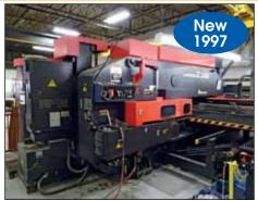
AMADA VIPROS Z358PPC 30-TON HYDRAULIC CNC TURRET PUNCH PRESS
