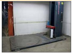
WULFTEC ROTARY STRETCH PALLET WRAPPER MODEL WLP-200
