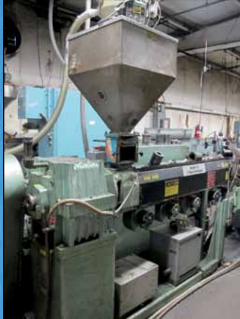
2.5" Davis Standard Extruder, 40 HP, Model MV-251N25, Mark VI,
