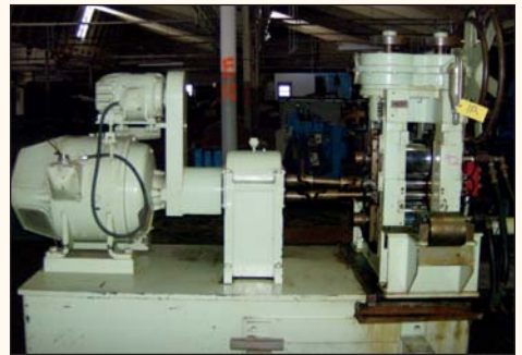
Waterbury Farrel 1.5" x 8" x 6" 4-High Rolling Mill, 20 HP
