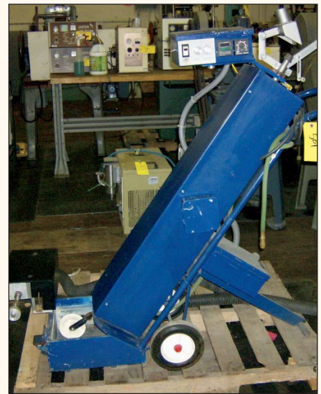
Goyette Vertical Chain Annealer w/ Atmosphere and Traverse Winder
