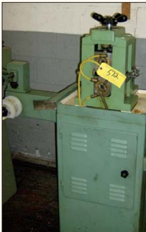
1271 MGS Carbide Rolling Mill w/Traverse Takeup
